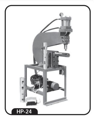
Throat Depth: 24 inches Capacity: 12 tons Stroke: 2 inches Cycle time round trip: Two stage pump (no load) 22/min Hydraulics: 2000 p.s.i., Bi-directional Electrics: 115VAC – 20 amps Controls (115 VAC): Double guarded foot switch Shut height: 6" Stand: Angle iron
