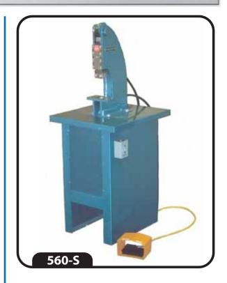
Combines in one machine, an ironworker, punch press, bender, angle shear, flat shear, "V" notcher, corner notcher, forming press, arbor press and pipe notcher. One model serves all operations. Because hydraulic power is delivered over the entire stroke, shearing action is built into tools and many cuts beyond the 560-S' rated 12 tons are possible with this amazing machine.
