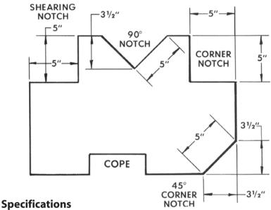
Capacity in mild steel 11 ga. Capacity in stainless steel 14 ga. Maximum notch in one cut 5''x 5'' Handle length 24'' + 6
