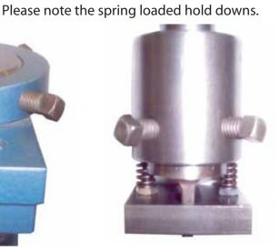
All the tooling shown above uses standard kidder punch and die holders.
