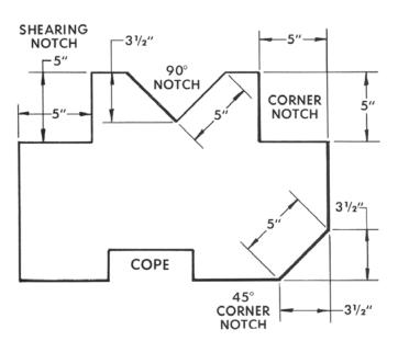
Note: Minimum length of cope determined by thickness of material. Coping is done in two stokes, turning blank.
